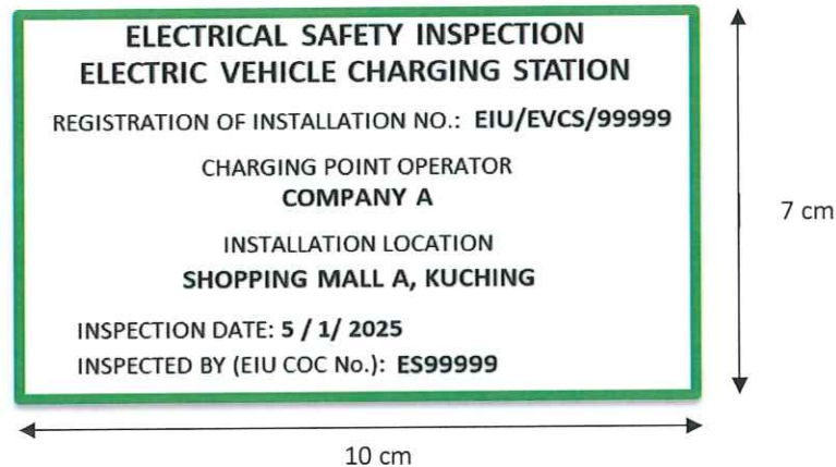
Figure 12: Electrical Safety Sticker
