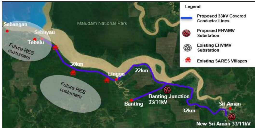
Figure 6: Extension of 33kV Covered Conductor Lines from Lingga to Sebuyau Along the Second Trunk Road
