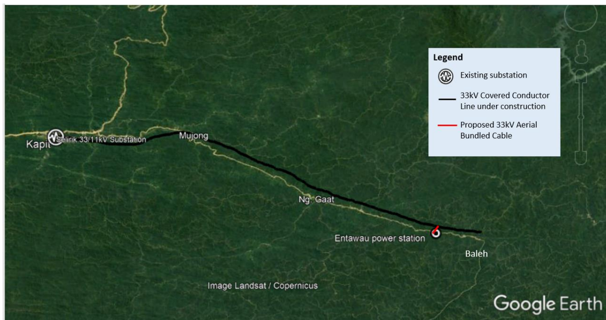
Figure 25: Tapping Selirik - Baleh 33kV Covered Conductor Line to grid-connect Entawau
