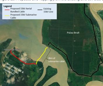
Figure 19: Proposed Line Tapping from the Existing Line at Pulau Bruit
