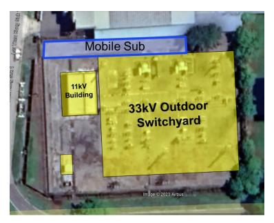
Figure 4.2: Proposed Location for mobile substation
